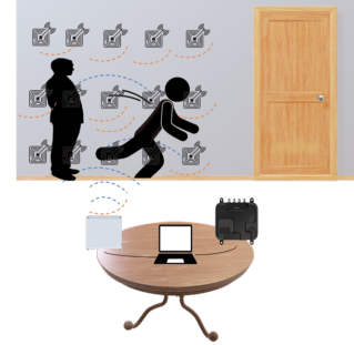
Figure 1: Experimental setup for data collection in a mock room to detect falling activity using Tag Array.
