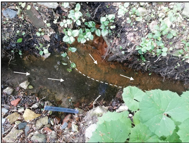
Fig. 8. Meeting of two discharges from 5 m apart. Discharge 2C (from the left) has a channel base with mostly organic matter, whereas Discharge 2B (from top of image) coats the channel base in orange ochre; 30 cm ruler for scale.
