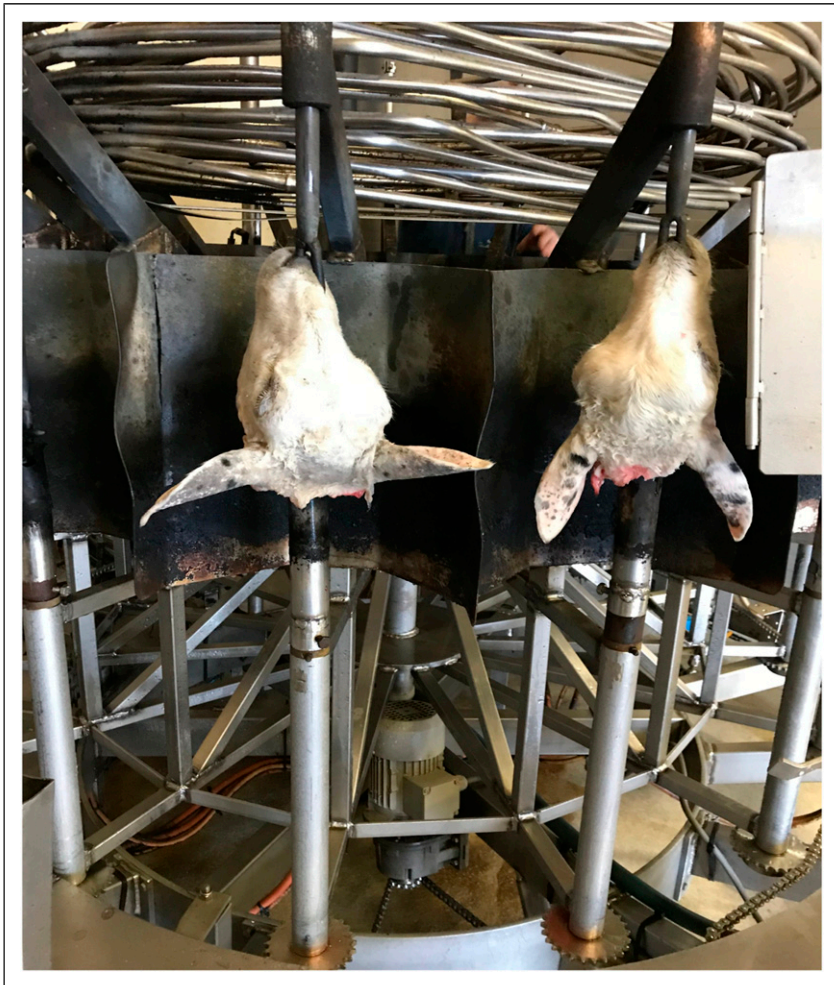
Figure 2. The mechanical sheep's head rotisserie.
