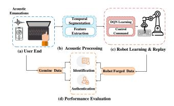
Fig. 1. Robot mimicry attack framework
