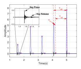
Fig. 2. Keystroke acoustic signal
