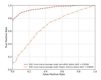
Fig. 8. The ROC curve under different attacks, i.e., zero-knowledge human attack and robot mimicry attack
