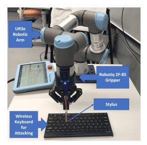
Fig. 3. The robotic arm typing on the keyboard
