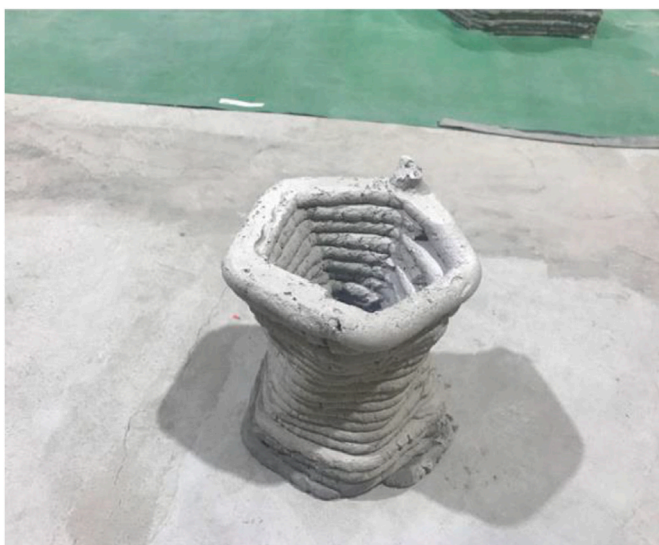
Fig. 10. MKPC sample used for 3D printing (reproduced from Ref. [154]).
