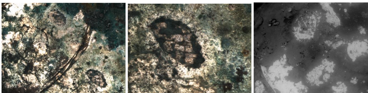
Fig. 22. a, b, and c: Photomicrographs and SEM BSE of the ghost textile surface on the silver frame encasing the rock crystal sphere (71.4); seen as light-coloured patches by SEM BSE (Image © National Museums Scotland).
