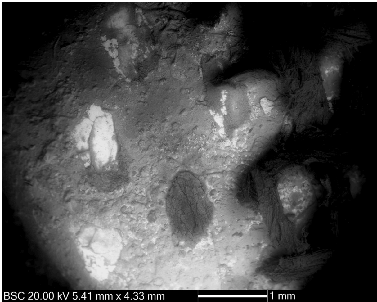
Fig. 10. SEM BSE image of the corroded area on the casing of the composite bead (71.5). The darker petal shapes are surviving organic threads - remnant textile surfaces; the lightest petal shapes are uncorroded silver - ghost textile surfaces (Image © National Museums Scotland).
