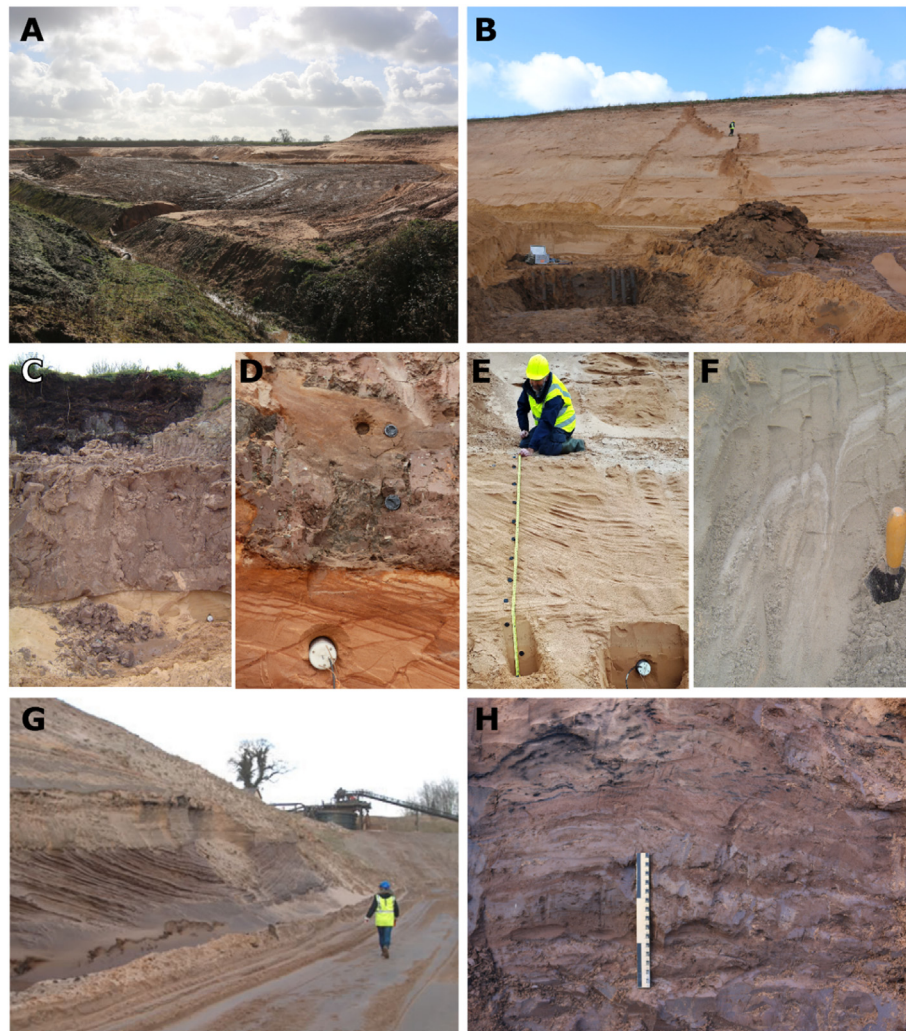
Fig. 3. Sedimentary units and bedding structures observed within the Arclid Quarry. (A) View of quarry workings at Arclid as of 2019. (B) Chelford Sands extending down to Oakwood Formation till (bottom right). (C) Stockport Formation till with Holocene peat filled kettle hole above and upper part of Chelford Sands below. (D) Close-up of interface between Stockport Formation till and luminescence samples (Shfd18098-99) in it and Chelford Sand with gamma spectrometer denoted luminescence sample Shfd18097. (E) Cross-cutting bedding within Chelford Sands with position of luminescence sample Shfd18147. (F) Syngenetic ice wedge cast within Chelford Sands. (G) Cross-section of channel fill in Chelford Sands. (H) Close up of the Oakwood Formation till at base of exposed stratigraphy.
