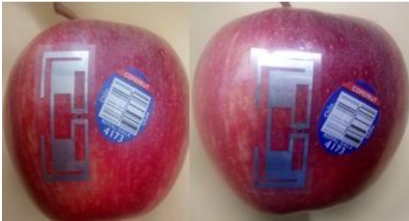
Fig. 9. Fabricated prototype of apple tag on two different apple samples.
