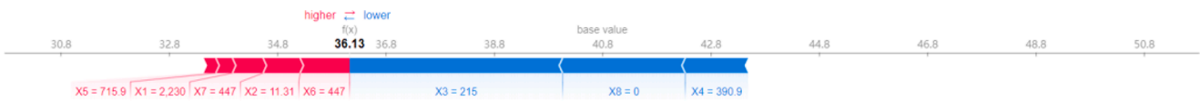
Fig. A6. Local multiple force interpretation diagram based on XGBoost algorithm ( X_1 : density, X_2 : cement content, X_3 : water content, X_4 : water absorption, X_5 : natural fine aggregates, X_6 : recycled coarse aggregates, X_7 : natural coarse aggregates, and X_8 : superplasticizer).
