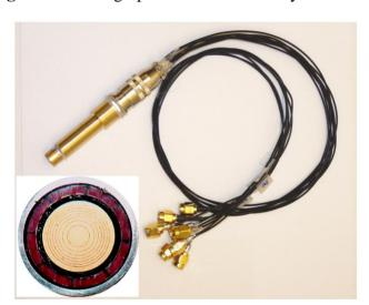
Figure 23. Photograph of the annular array transducer.
