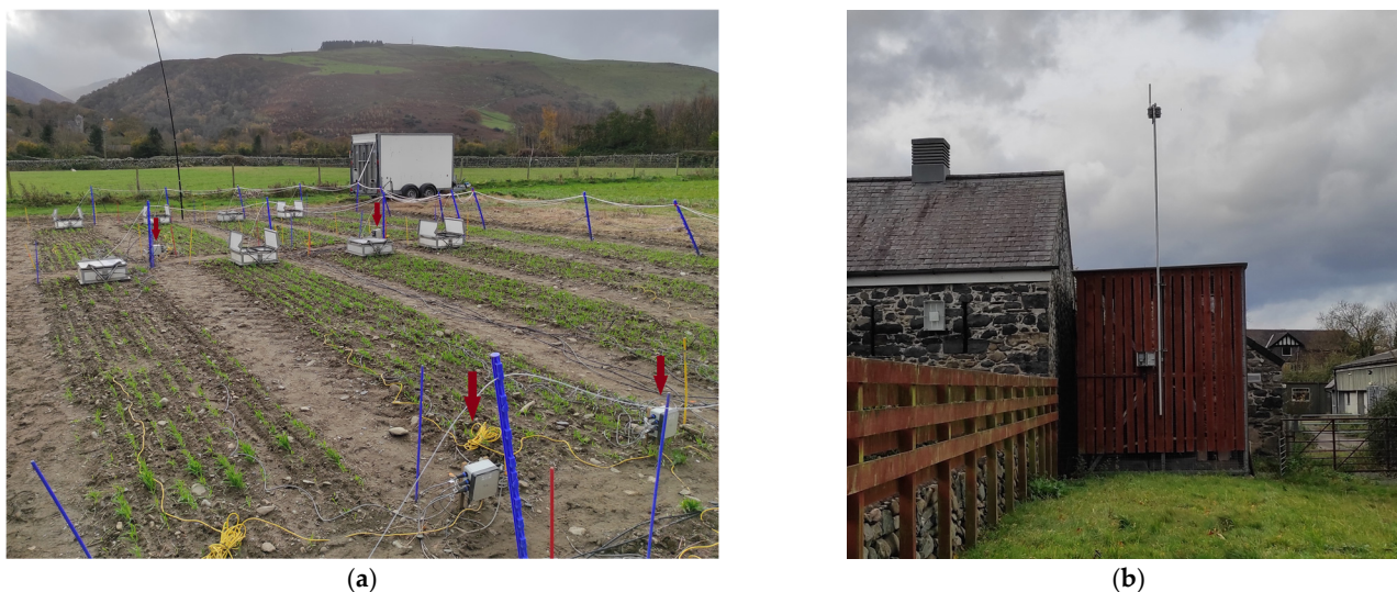
Figure 10. Deployment at Henfaes Research Farm, Abergwyngregyn: (a) nodes (arrowed) deployed in a wheat crop (the large, lidded boxes are measuring greenhouse gases); (b) MultiTech LoRaWAN gateway.
