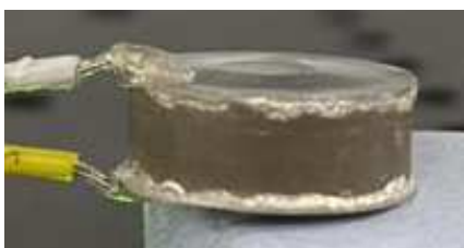
Fig. 2. The Nitinol cymbal device, where device components can be identified using Fig. 1 for reference.
