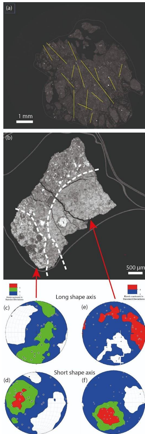
Figure S16. Example XCT data from Winchcombe meteorite samples BM.2022,M1-84 and BM.2022,M2-34. (a) and (b) – Example CT slice from two samples, with (a) showing aligned fractures and (b) showing three distinct lithologies distinguishable by their texture and contrast variations. (c) and (e) – lower hemisphere projection of the long shape axis of chondrules showing a weak-moderate girdle fabric. (d) and (f) – lower hemisphere projection of the short shape axis of chondrules showing a weak-moderate lineation fabric. Their preferred alignments in the long and short shape axis of chondrules are consistent with a foliation fabric caused by compaction.
