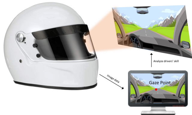
Fig. 1. A schematic diagram of the eye tracking racing helmet
