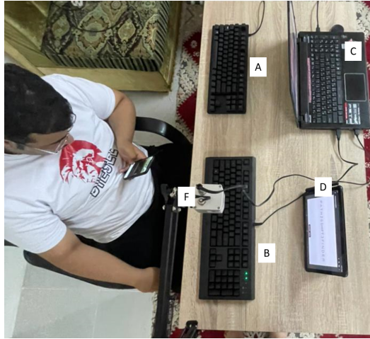
Fig. 15. An example of a session from Study II: In every session, the thermal camera (F) was mounted on a tripod at varying heights and distances from the keyboards. (A) a Razer Huntsman Tournament Edition gaming keyboard (PBT keycaps). (B) a Razer Cynosa Lite Gaming Keyboard (ABS keycaps). The content participants should type was shown to the participant on Laptop1 (D), while the experimenter recorded the thermal images using Laptop2 (C) which was connected to the thermal camera.
