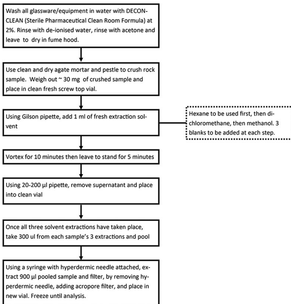
FIG. 1. Solvent extraction protocol carried out to capture a broad range of solvent-soluble metabolites in meteorite samples. All steps were carried out at room temperature ( \sim 20^{\circ}\text{C} ).
