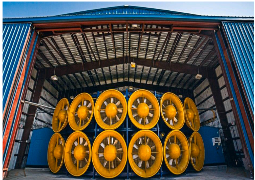
Figure 10. NHERI Wall of Wind Experimental Facility [24].
