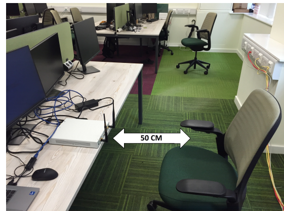
Fig. 3: Experimental setup of USRP placement with chair
