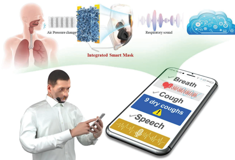
Figure 1. The application of smart masks for monitoring human daily respiratory activities.
