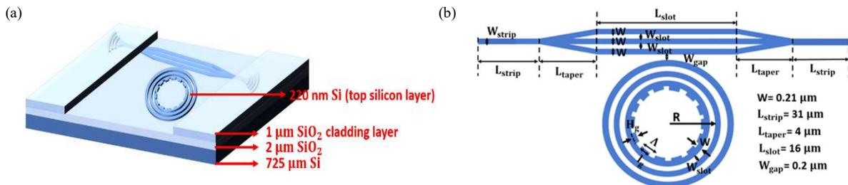
Fig. 1. (a) Schematic structure of the IG-DSMRR, (b) Detailed design parameters of the IG-DSMRR structure.
