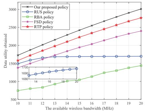
Fig. 3. Data utility obtained vs. the available wireless bandwidth
