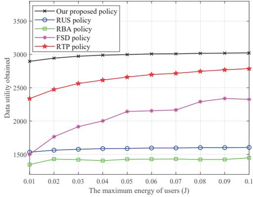
Fig. 4. Data utility obtained vs. the maximum energy of users
