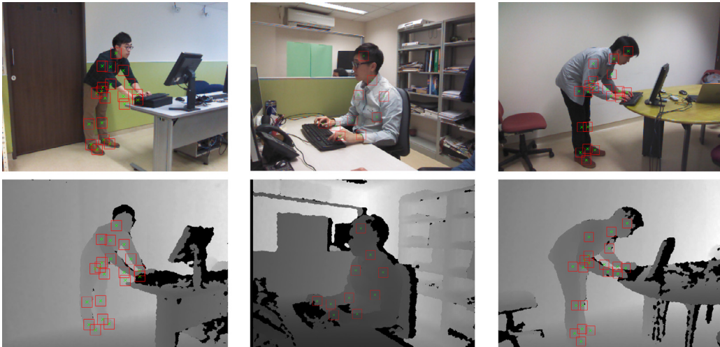
Fig. 2. Examples of image patches (shown in red squares) extracted around the body joints for computing the color and depth images reliability terms. Mis-tracked joints such as the left elbow (in the middle column) result in large difference in the patches. (For interpretation of the references to color in this figure legend, the reader is referred to the web version of this article.)
