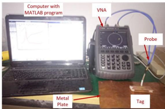
Fig. 14. Impedance measurement setup using Vector Network Analyzer and two-port Probe
