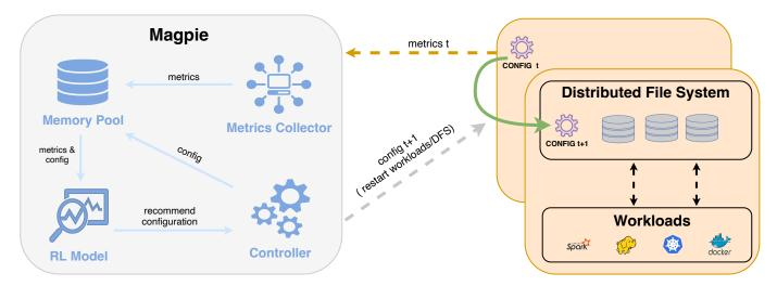
Fig. 1: General idea of Magpie. The left side presents the four main components of Magpie and the right side illustrates the distributed file system (DFS) and workloads running on it. Magpie collects metrics for a given configuration t and then analyzes its execution history to recommend a new configuration t + 1 to the DFS. Both the DFS and / or the workloads will then be restarted to apply new configurations.
