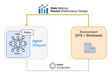
Fig. 2: RL problem representation. Each component is illustrated with its role. The agent (Magpie) interacts with the environment (DFS + workloads) by collecting the state (metrics) and reward (performance gains) and taking actions (applying new configurations).
