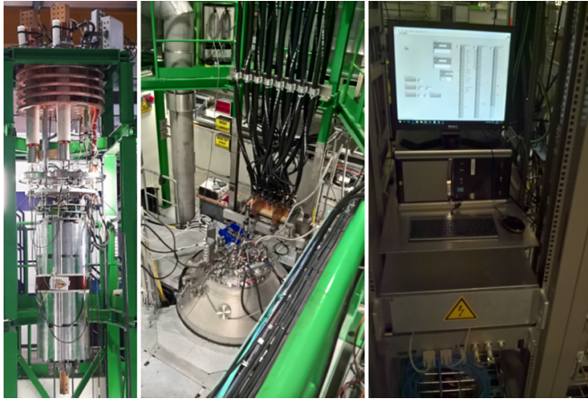
Figure 11. Test facilities for testing quadrupole magnet [106].
