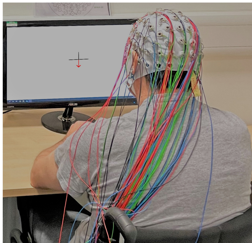
Figure 2. Setup for EEG recording. The downward arrow is the cue to perform motor imagery of the legs. The picture was taken with written consent from the participant.
