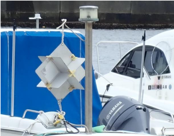
Figure 1. Photograph of an 8 corner-reflector on a small boat.
