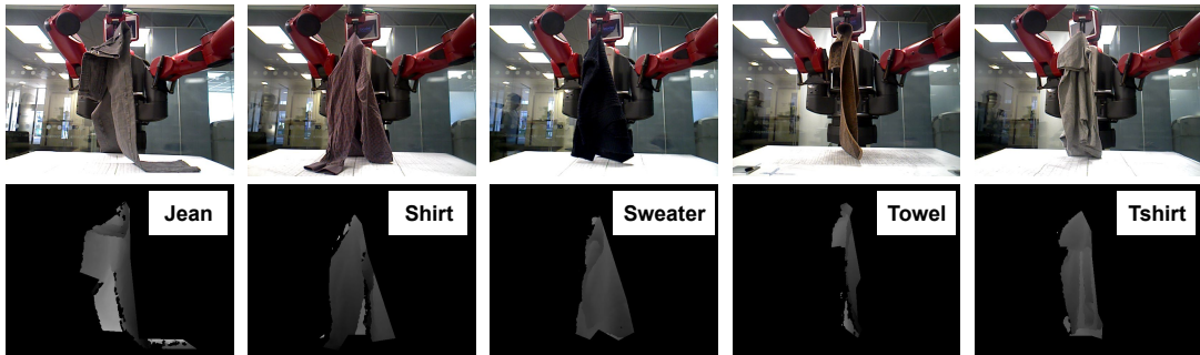
Fig. 2. Database Examples : There are five garment categories in our database: jeans, shirts, sweaters, towels and tshirts. Our database contains masked depth and RGB images of four garment instances in each category, which have five categories (Top: original images, Bottom: masked depth images).
