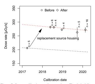
Figure 7. Source-calibration results over time. The dashed lines indicate the predicted dose-rate evolution of the  $^{90}\mathrm{Sr}/^{90}\mathrm{Y}\text{-source}$  based in the first calibration point. The circle indicates the dose rate before, the diamonds the dose rates after the source housing was replaced. Dose-rate values refer to calibration measurements under the source with its shutter closed. Shown are mean  $\pm$  standard deviation of the mean.
