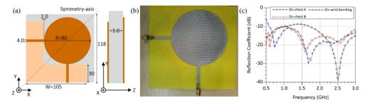
**Figure 1.** The proposed e-textile sensing antenna: (**a**) layout and dimensions (in mm); (**b**) photograph of the fabricated prototype; (**c**) measured reflection coefficient of the antenna on different body parts showing a matched impedance.
