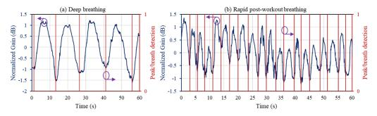
Figure 3. Successful breath rate measurement using a peak-detection algorithm.
