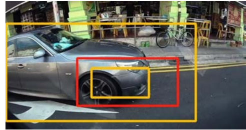
Fig. 5: Illustration sample of “minimal illegal units”. The rectangle in red is the acceptable “minimal illegal units” and rectangles in orange are other defective units.
