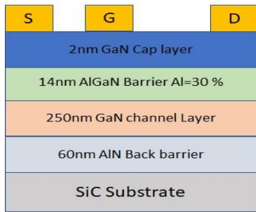
Figure 1. Schematic diagram of fabricated buffer-free AlGaN/GaN HEMT structure. The total thickness of the epitaxial layers is only 326nm.
