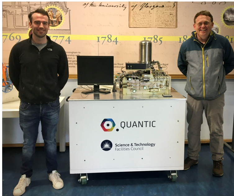
Figure 1. The viewpoint authors with a compact cryogenic system for SNSPDs, as reported by Gemmell et al. SUST 2017 [25].
