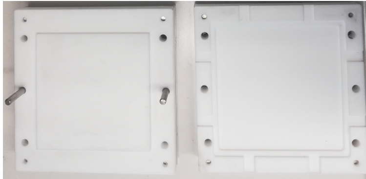
Fig. 4 unfilled sample molds used for the preparation of silicone samples intended for electro-mechanical testing.
