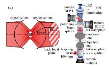
FIG. 1. (a) Schematic sketch of the electromagnetic field E(x, y) arising from the interference of incident and scattered light, which is used to calculate the optical torque acting on the trapped particle. (b) Experimental setup.
