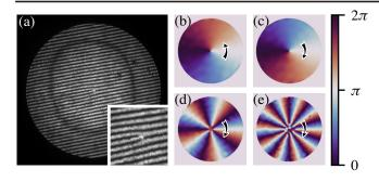
FIG. 2. Results for field retrieval for beams with a spiral phase  $\exp(il\varphi)$ . (a) Observed interference pattern for l=+1. Inset: characteristic fork shape at the center. (b) Retrieved phase for l=+1, (c) for l=-1, (d) for l=-5, and (e) for l=-10.
