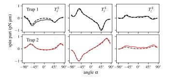
FIG. 4. Simultaneously measured spin torque (solid lines) and sequentially measured torques with a single trap (dashed lines) for each microsphere of the dumbbell object.
