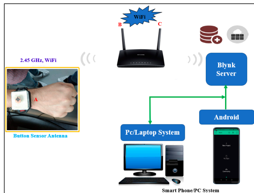
Figure 2. Design system architecture for the button sensor antenna (Point A: BSA Device, and Points B, C: WiFi Router).
