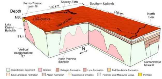
629 Fig. 4: A schematic illustration of our 3D geological model. Carboniferous basin structure after
