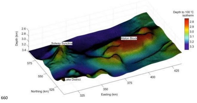
661 Fig. 9: Modelled depth to the 100 °C isotherm.
