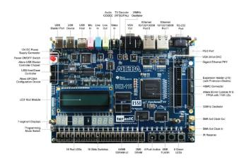
Fig. 2. Altera's DE2-115 FPGA board for teaching and research, the DE2 series FPGA development boards have long been acclaimed for their rich and diverse peripheral interfaces, and have been the leading educational development platform and the first choice of laboratories in 1000 schools worldwide.
