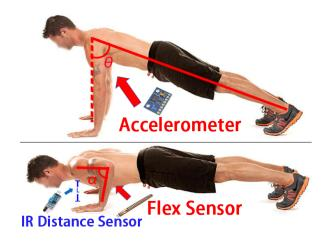
Fig. 6. Body position measured by different sensors.
