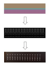
Fig. 4. Image processing result, from the input image to the theoretical output result to the actual output result, the edges of different colors are recognized and converted to ascii code.
