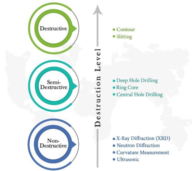
Fig. 2: Experimental techniques for assessing residual stresses.
