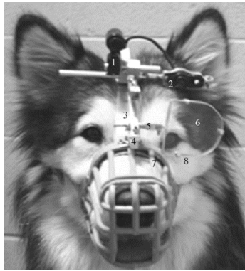
Figure 10. Using a head-mounted, eye-tracking system with dogs [110].
