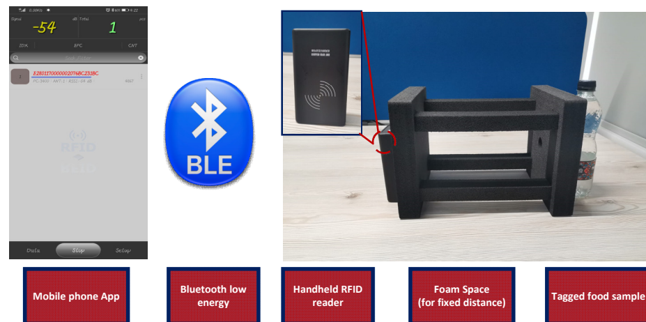
Figure 6. Handheld reader based setup connected with smart phone for food contamination sensing.
