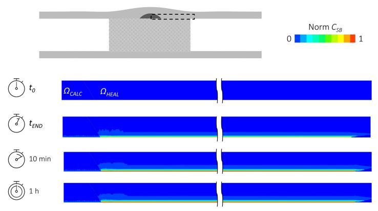
Fig 3. Spatial maps of normalized specifically-bound  $(C_{SB})$  drug concentration on the section along the main direction in the case of DCB inflation of 180 seconds. The temporal evolution is studied at 4 time instants: the beginning  $(t_0)$  and end  $(t_{END})$  of the DCB inflation, at 10 minutes (10 min) and 1 hour (1h) after DCB deflation. The location of the color maps is indicated at the top of the schematic.
