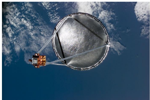
Fig. 1. 14 m diameter Inflatable antenna experiment STS-77 1996 (NASA)
