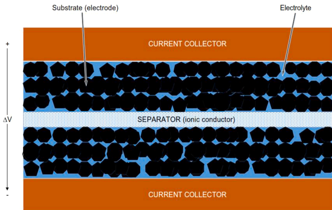
Fig. 42. Architecture of a supercapacitor González et al. [110].
