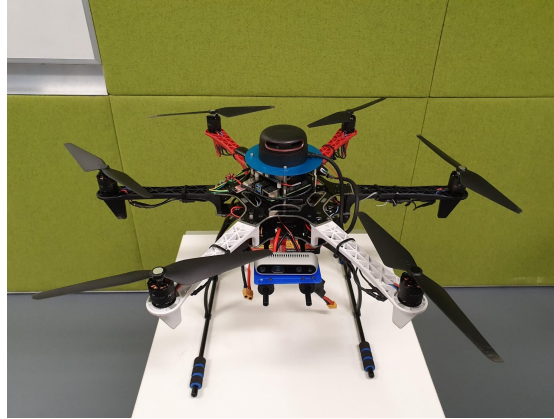
Fig. 2. Our drone configuration with integration of RPLidar A2 (bottom left) and Intel RealSense D435i (bottom right).
