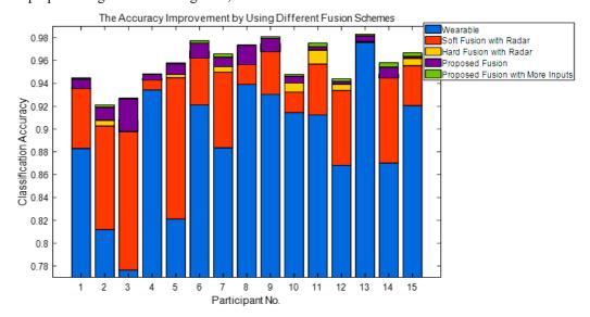
Fig. 3. From [21]: Accuracy obtained by Bi-LSTM network classifier for continuous sequences of human activities using multimodal inputs, namely data from wrist-worn wearable (blue) fused with descriptors derived from radar spectrograms (different colours). The results are presented for each participant considered as unseen test subject to validate the classifier's performances (Leave One Person Out validation approach)
