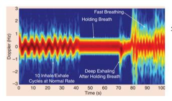
Fig. 2. Inspired from [1]: Radar spectrogram for a person sitting on a chair at approximately 60 cm from the radar and simulating different respiration rates and patterns. Specifically, the subject was asked to perform 10 cycles of normal respiration followed by a long period of holding breath and then fast, accelerated breathing. The radar used for this tes operated in the X-band, within the Ultra Wide Band (UWB) spectral region.
