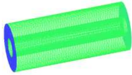
(a) Inlet and Outlet Grids (Structural Grids)
