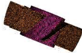
(b) Impeller Grids (Unstructured Grids)
