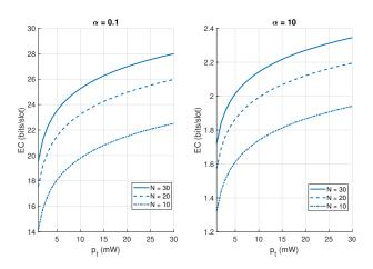
Fig. 6. The impact of the number of IRS elements (N) on the EC of the MISO downlink for the case of no CSI at the BS: delay-tolerant communication regime (left), delay-limited communication regime (right).
