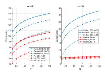
Fig. 7. The impact of the number of transmit antennas  $(N_t)$  at the BS on the EC of the MISO downlink: delay-tolerant communication regime (left), delay-limited communication regime (right).
