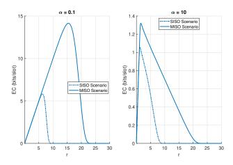
Fig. 8. The EC turns out to be a concave-like function of the transmission rate r. (The sub-plot on the left depicts the delay-tolerant communication regime, while the sub-plot on the right depicts the delay-limited communication regime.)
