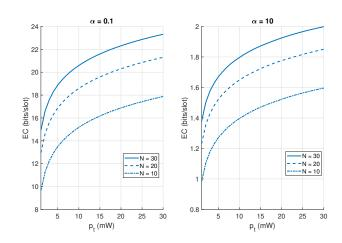
Fig. 4. The impact of the number of IRS elements (N) on the EC of the SISO downlink for the case of no CSI at the BS: delay-tolerant communication regime (left), delay-limited communication regime (right).
