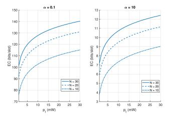
Fig. 3. The impact of the number of IRS elements (N) on the EC of the SISO downlink for the case of perfect CSI at the BS: delay-tolerant communication regime (left), delay-limited communication regime (right).
