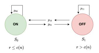
Fig. 2. Markov chain representation of the IRS-aided SISO downlink for the case of no CSI at the BS.
