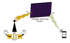
Fig. 1. The system model: we examine the QoS performance of a downlink channel whereby a panel of N passive, reflective IRS elements assists the communication between the BS and the UE. A(t), S(t) represent the arrival process and the service process at the BS queue, respectively.
