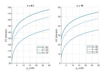
Fig. 5. The impact of the number of IRS elements (N) on the EC of the MISO downlink for the case of perfect CSI at the BS: delay-tolerant communication regime (left), delay-limited communication regime (right).
