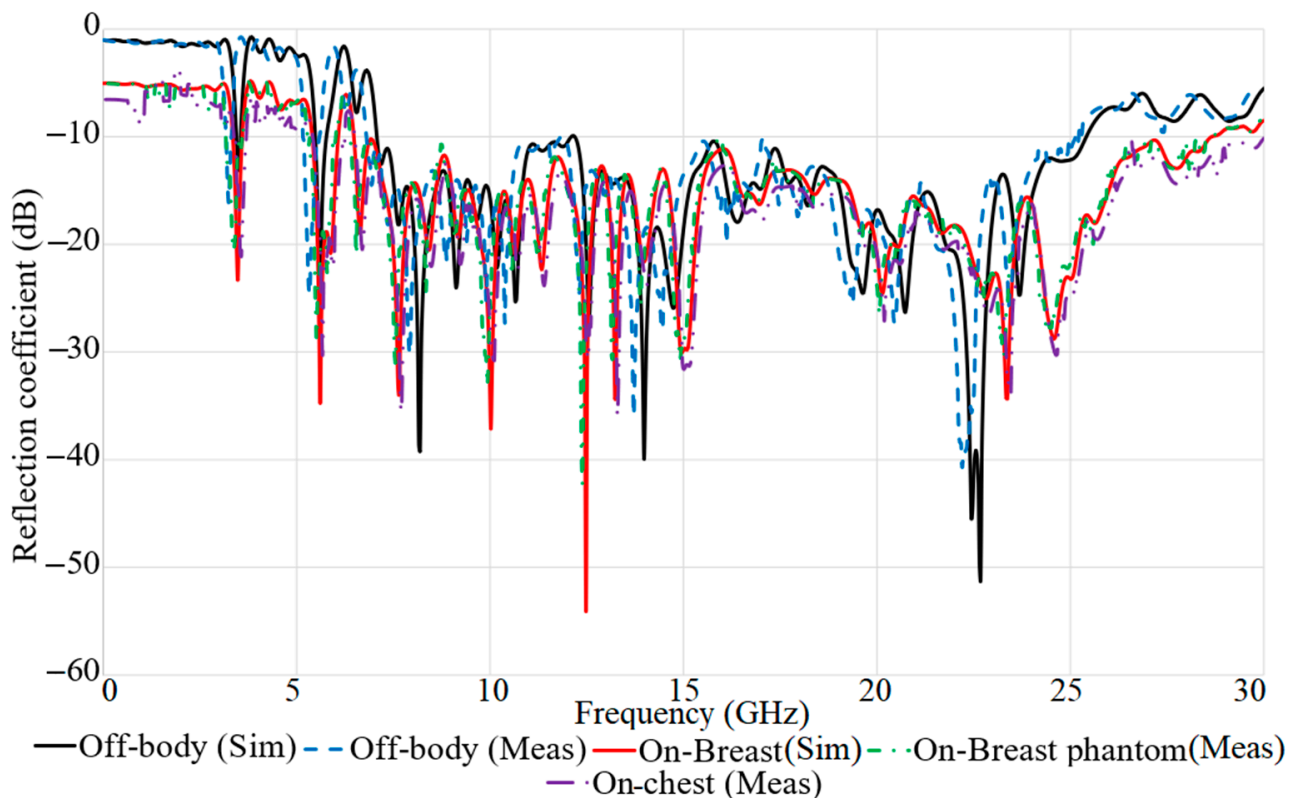
Figure 4. The reflection coefficient result of the proposed antenna on-body (on breast) and off-body for simulation (sim) and measurement (meas).
