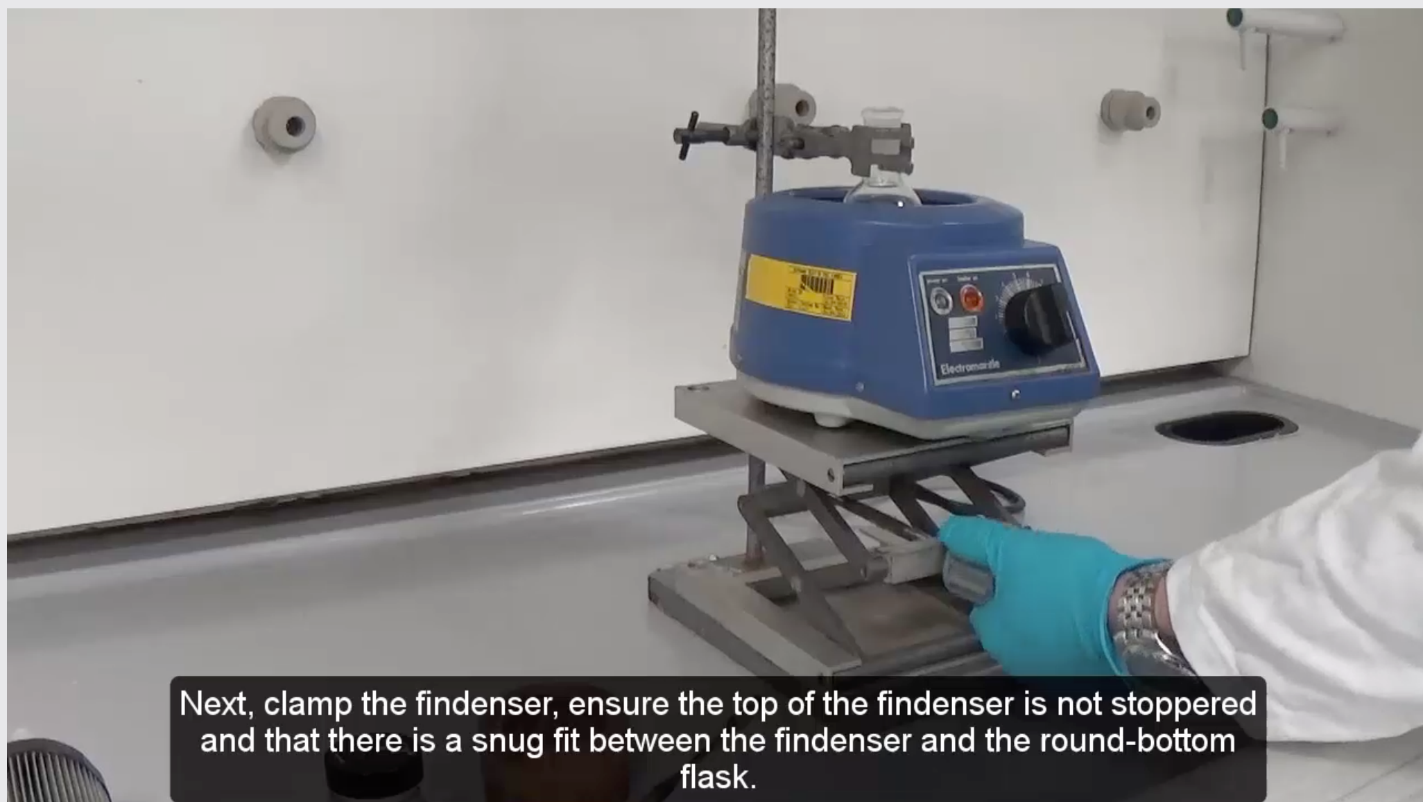
Figure 2 – Reflux technical film (excerpt) with audio (Jarrett Gray), showing subtitles and tip / safety call-outs to draw student attention to potential challenges and safety issues.
